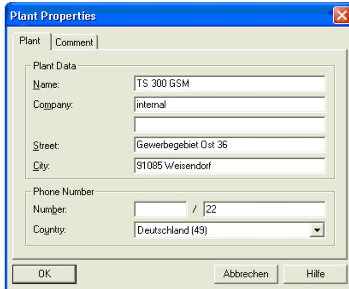
System or network-specific settings of the SSW7-TS with GSM modem can be made with the TeleService software or SHTools (see chapter 4.3.3 ).
